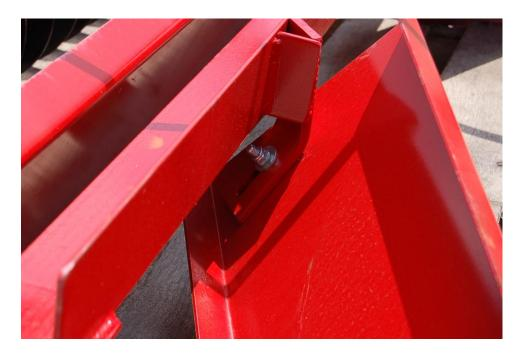
Front shaping board adjustment holes. In the front, at leading edge.
