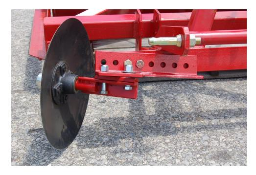
If the disks are worn and need to go deeper than the brackets allow, spacers can be placed between the disk mount angle iron with the vertical bolts and the disk to 3 point hitch angles (the ones that are adjustable from side to side.
