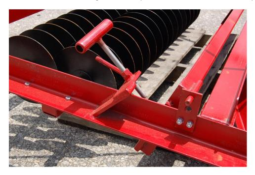
Front shaping board adjustment holes. In the center, at trailing edge.
