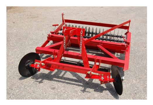
The shaping boards in the front behind the disks, are adjustable for the width of the bed top you are trying to achieve. The lower the leading edge, the more soil it will capture. The higher the trailing edge, the wider the bed will be.
