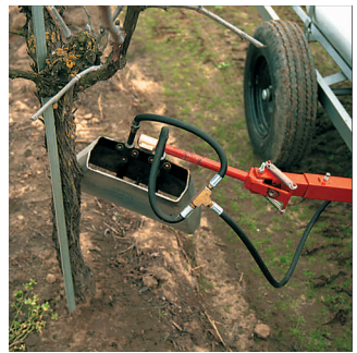
All GP flamers feature a spring loaded break-away boom arm system so there is no worry about damage to the vine, tree or equipment. The arms immediately snap back into operating position once it has passed.
