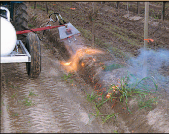
Flaming applies intense heat to weeds and grass causing the cell structure of the plant to be destroyed. You do not have to burn weeds to a crisp.
