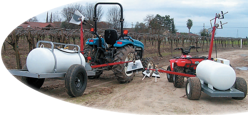
All GP flamers feature a spring loaded break-away boom arm system so there is no worry about damage to the vine, tree or equipment. The arms immediately snap back into operating position once it has passed.
